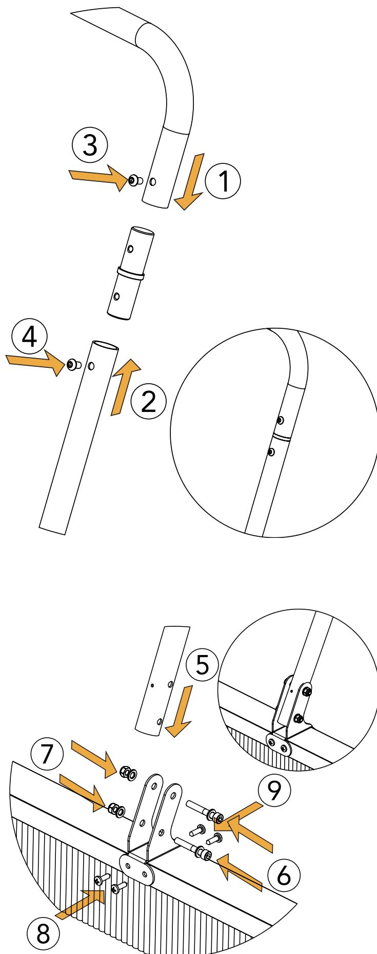
1. Install the DHANDLE onto the HANDLE JOINER, ensure the hole in the DHANDLE lines up with the hole in the HANDLE JOINER
